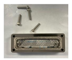
7. Wipe the "O"-ring and "O"-ring mating surface with a clean lint-less wipe.
