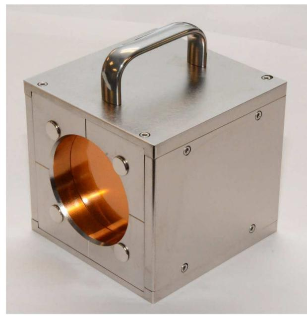
Prototype MLFC assembly with 128 layers of 0.0508 mm copper, suitable for proton beam energies up to 250 MeV. The assembly weighs 5.6 kg (12.2 lb) and measures 120 x 120 x 145 mm. The sheets are fully screened inside the housing and the signals are brought out on two VHDCl68 connectors. The useful area is 72 mm diameter, sufficient for the beam size of most PBS systems.
