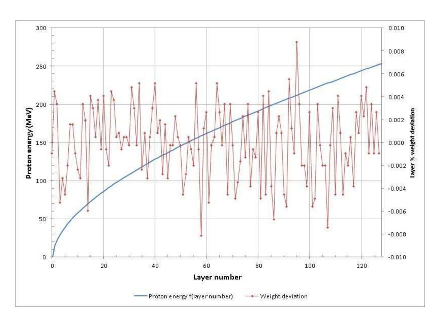
Relationship between MLFC layer number and proton energy for the prototype MLFC which is stored as a device-specific table. The weight deviation curve illustrates the corrections applied in the creation of the table.
