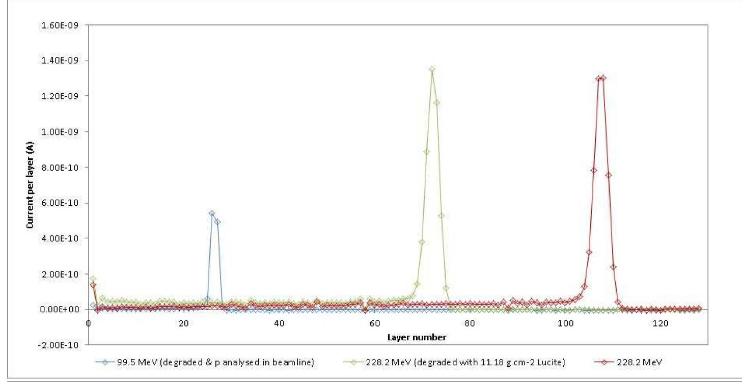
Raw data for three different beam energy conditions. The low-energy tails are the result of nuclear scattering secondaries.
