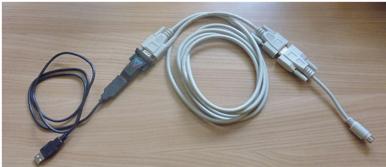
Figure 8. RS-232 connection arrangement using USB and mini-DIN adaptors.
