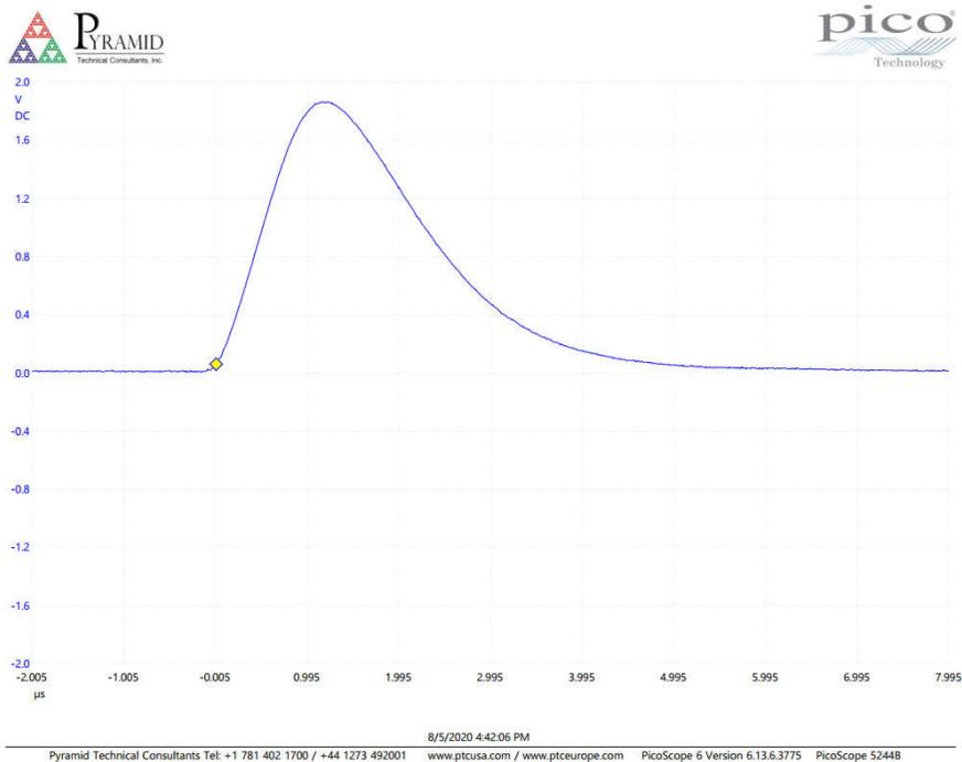
The classic solution is to first integrate the charge, then use a shaping amplifier to form a clean pulse whose height represents the amount of charge. The Pyramid CR-10 product uses this approach. The pulse shown below is the result of a 1  $\mu$ sec shaping time constant. The CR-10 allows flexibility in choice of shaping time constant and a wide range of gain settings. It is physically larger than the CP-10 or CP-15.
