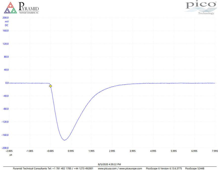
The CP-15AF provides additional gain and optional inversion of the signal. Higher gain allows the photomultiplier bias voltage to be reduced, giving lower background dark count rate.
