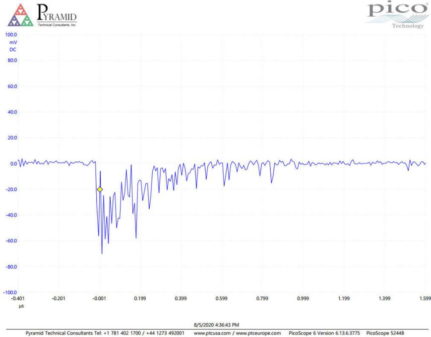
Such a signal is clearly unsuited to either pulse counting or pulse height analysis. A lower bandwidth preamplifier like the CP-10A is a good choice for fast scintillation detectors, but still reveals too much detail in a NaI detector output.
