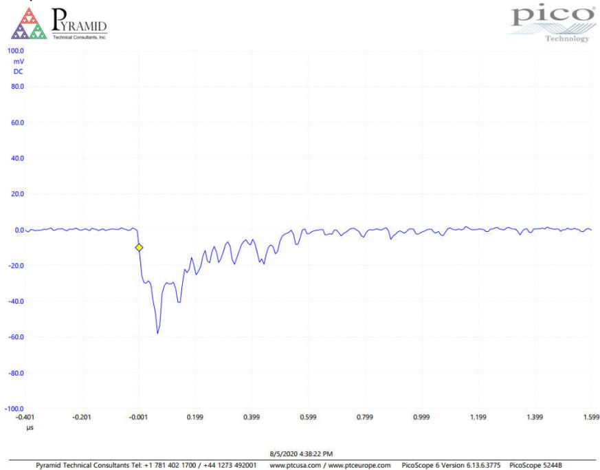
The Pyramid CP10AF preamplifier adds filtering to eliminate the detailed time structure and leave a single clean pulse.
