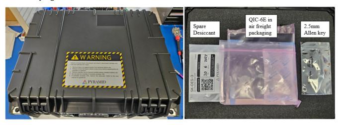
2. Remove the IC from the bag and completely remove the 4 screws on the desiccant port cover using the 2.5mm Allen key.
