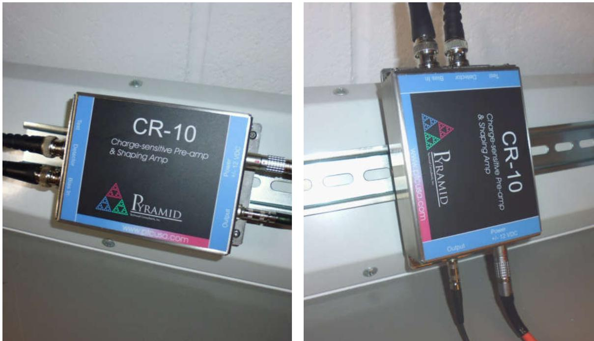
Figure 4. DIN rail mounting.
