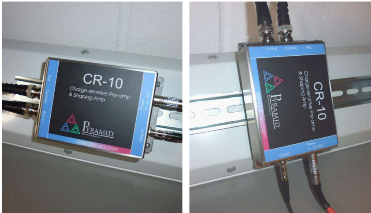
Figure 4. DIN rail mounting.
