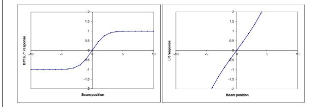
Similar position functions can also be used for broad beams such as passively scattered proton therapy beams, in which case they indicate beam flatness rather than centroid location.
