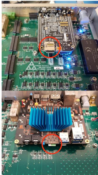
To remove the card gently press the card in like a button and it should then pop back out and be easily removed. To install a card do the same but in reverse were you gently press in to lock the card back into place.
