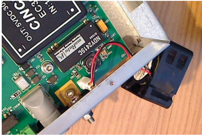
Figure 3 - Fan power connector (2 pin Molex)
