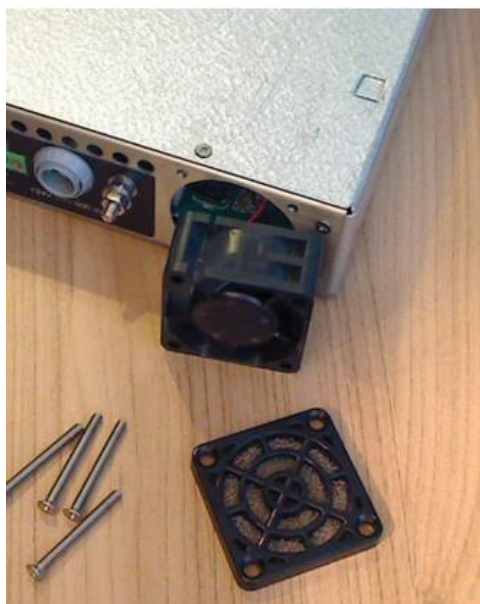
Figure 15 - Fan filter removal
