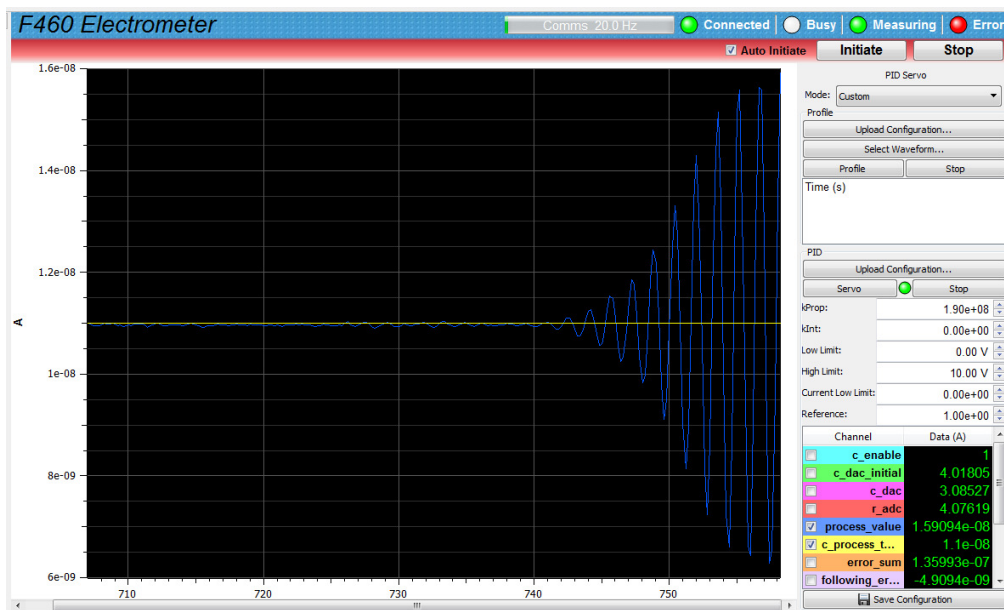
Figure 84. Oscillation when proportional term is increased.
