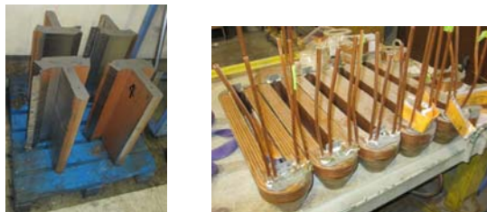
Figure 4. Lamination stacks and coils in manufacture for the prototype octopole magnet
