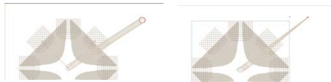
Figure 8. Ray trace simulations looking back along the beam axis: deflection only, and deflection plus quadrupole doublet focusing
