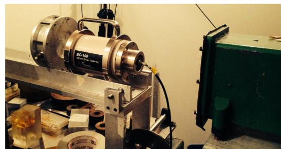
BC-100 beam collector under test at MGH. The dose control ion chamber and part of the reference NFC are visible. Sequential measurements were taken with the NFC, the BC-100 and an MGH beam collector.
