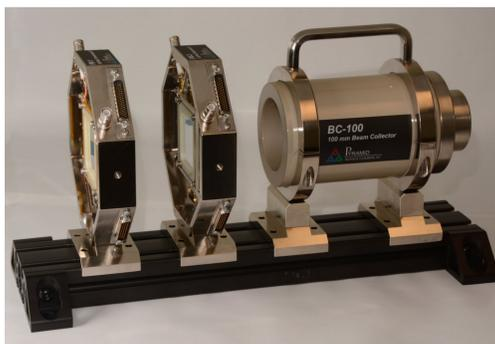
Assembly of two ion chambers and beam collector. Nominal position for the isocenter plane is equidistant between the chambers. The mechanical assembly is mounted on a motion system that can position it anywhere in the beam scan field on the isocenter plane. A optional gimbal arrangement allows it to be rotated to track gantry rotation.
