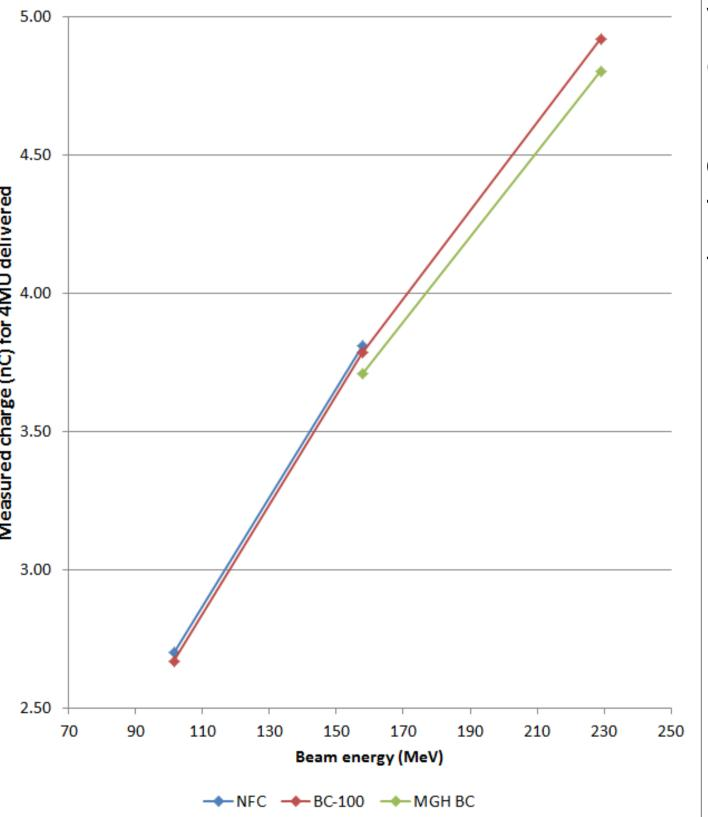
very small, however, only -0.62% at the highest energy accessible to the NFC. This is very promising for its use as a reliable absolute dose measurement device. The table shows the measured charge in nC for 4 MU delivered at three beam energies. NFC MGH BC Energy *BC-100* 101.5 2.669 2.699 157.8 3.808 3.784 3.709 229.0 4.803 4.919
