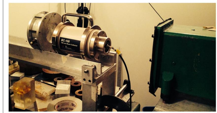
BC-100 beam collector under test at MGH. The dose control ion chamber and part of the reference NFC are visible. Sequential measurements were
