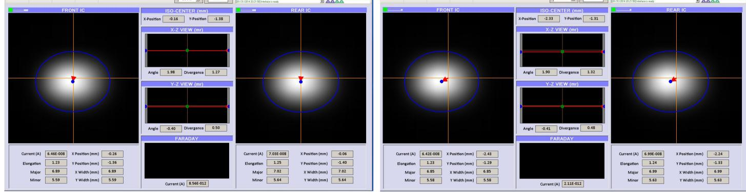
Successive screen shots showing detection of a beam shift of about half of the pixel size. The software allows the data to be logged to a local files or exported to EPICS [5]. A replay facility allows the user to step through a sequence of recorded measurements to look for transient effects.
