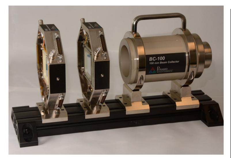
Assembly of two ion chambers and beam collector. Nominal position for the isocenter plane is equidistant between the chambers. The mechanical assembly is mounted on a motion system that can position it anywhere in the beam scan field on the isocenter plane. A optional gimbal arrangement allows it to be rotated to track gantry rotation.
