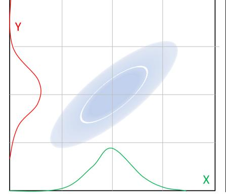
An inclined elliptical beam cannot be distinguished when viewed only as a projection onto X and Y axes. However such a beam may invalidate treatment planning assumptions, and therefore must be detected by any effective beam diagnostic system.
