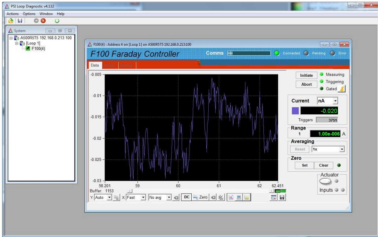
Figure 15. Data/current tab: F100 running with default settings, showing background noise
