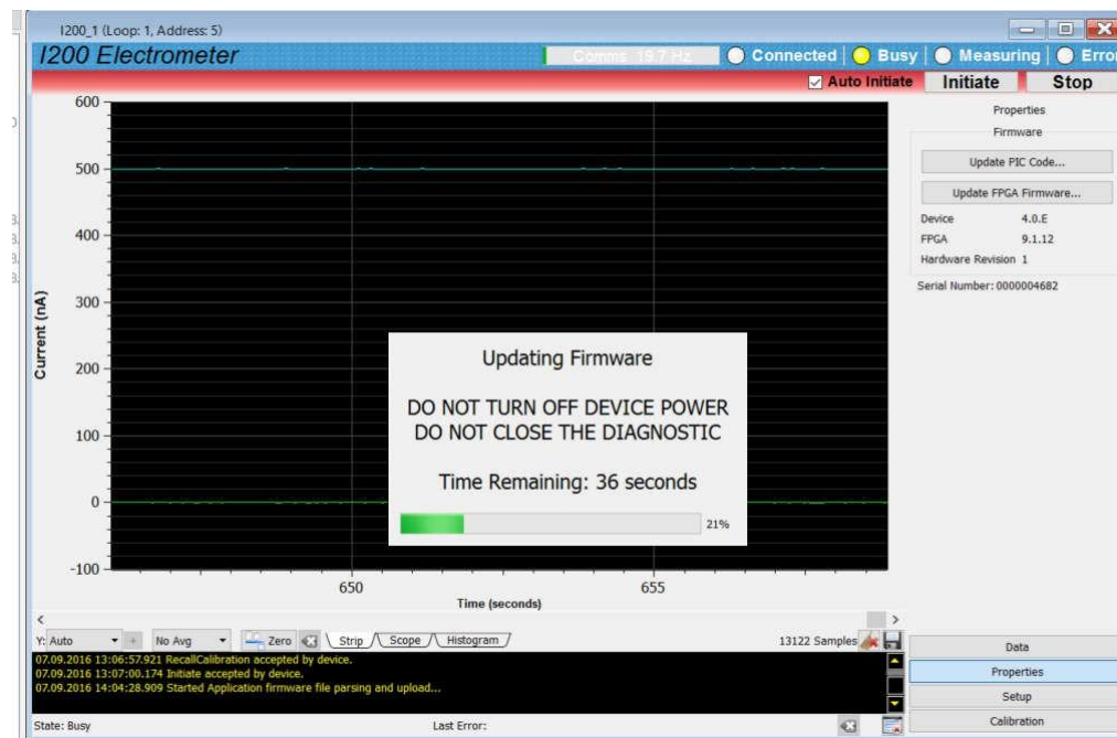
Figure 84. PIC firmware upload in progress (PTC DiagnosticG2).
