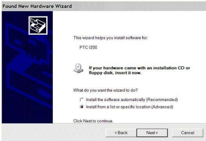
Figure 38. USB driver install step 2.
