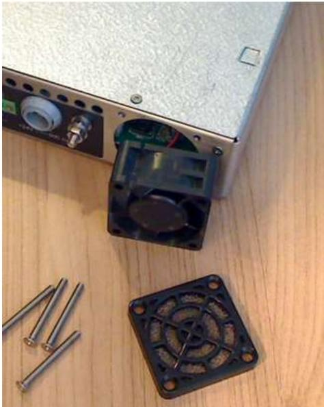
**Figure 16 - Fan filter removal**
