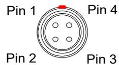
(External view on connector / solder side of mating plug)
