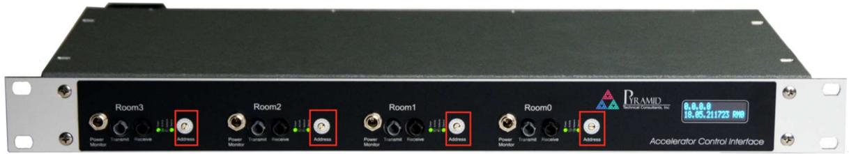
Figure 5 - Locations of M40 room interface loop address switches
