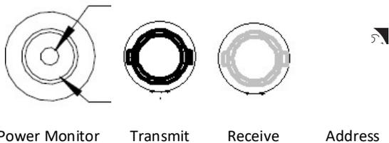
Two HFBR ST bayonets suitable for 1 mm plastic or 200  $\mu$ m silica fiber. 640 nm (visible red) light. Dark casing = receiver, light casing = transmitter.
