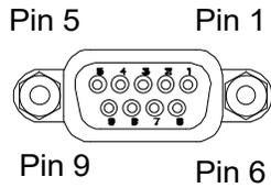
(External view on connector / solder side of mating plug)
