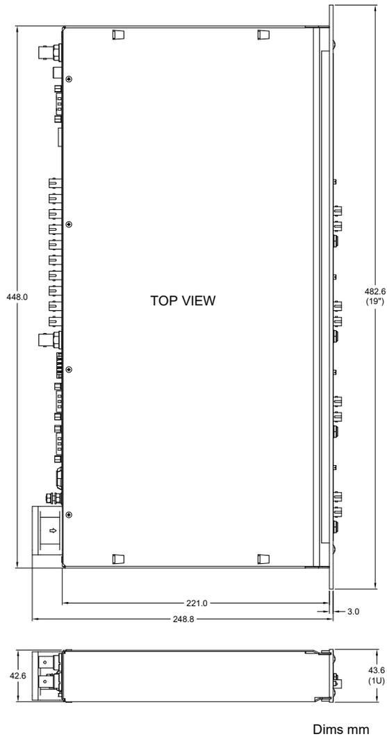
Figure 3 - ACI case plan and side views. Dimensions in mm.
