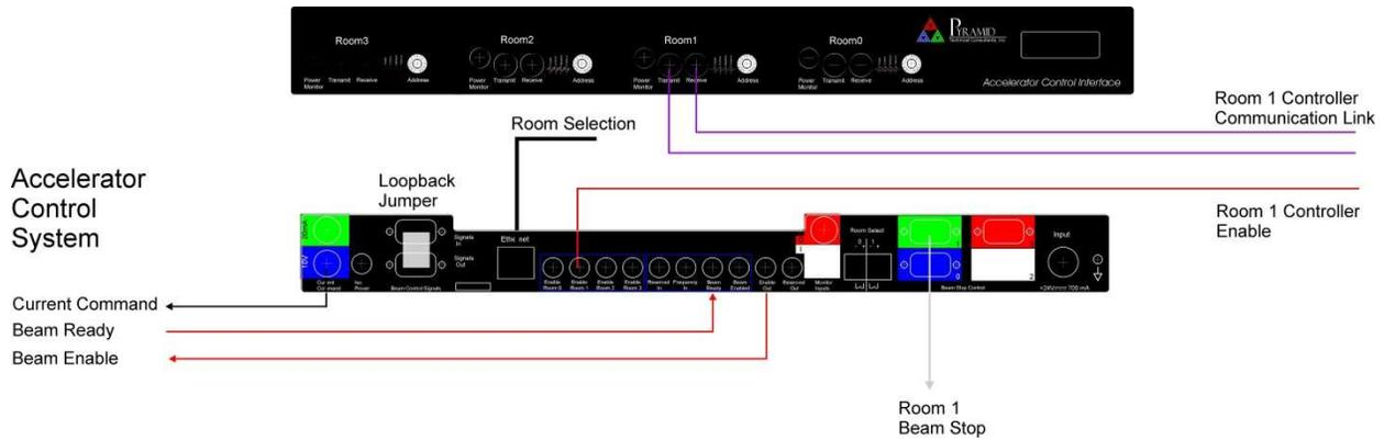
Figure 7 - Typical connections
