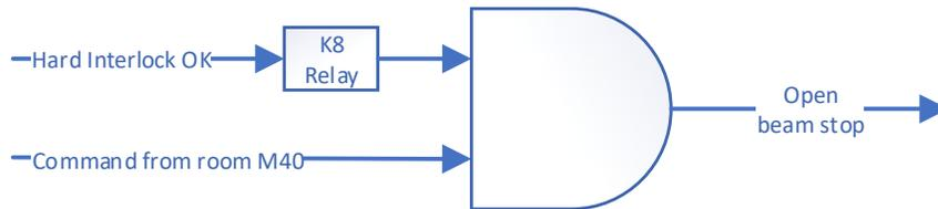
Figure 10 - Beam stop logic
