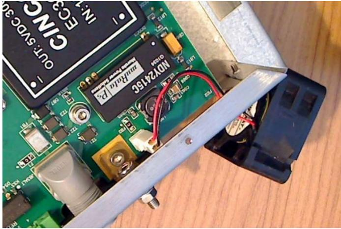
**Figure 17 - Fan power connector example (2 pin Molex)**
