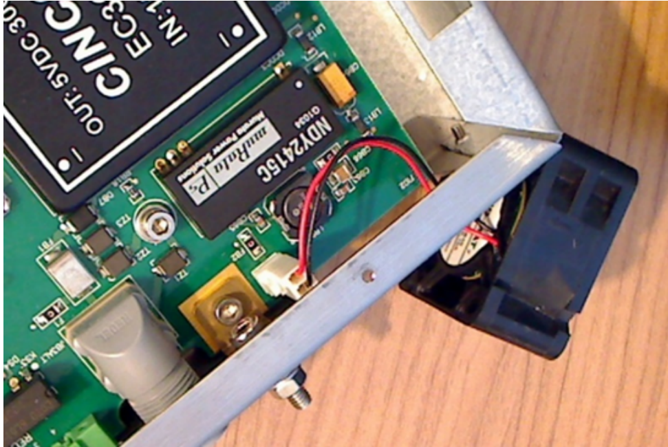
29 Fan power connector example (2 pin Molex)
