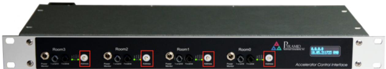
4 Locations of M40 room interface loop address switches
