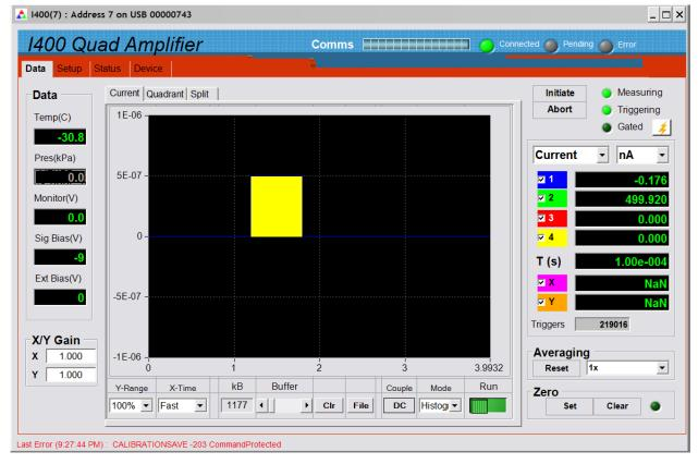
Figure 14. Internal calibration current routed to channel 2, histogram display format.
