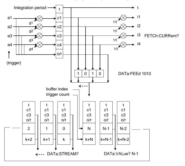
Figure 24. I400 data flow. The feed mask is set to pass data from channels 1 and 3.
