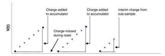
Figure 20. Illustration of integrator voltage at ADC sampling points during charge accumulation. The reset periods are shown relatively large.
