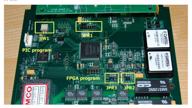
Figure 31. Internal switch and jumper locations. The screening cover has been removed for clarity.
