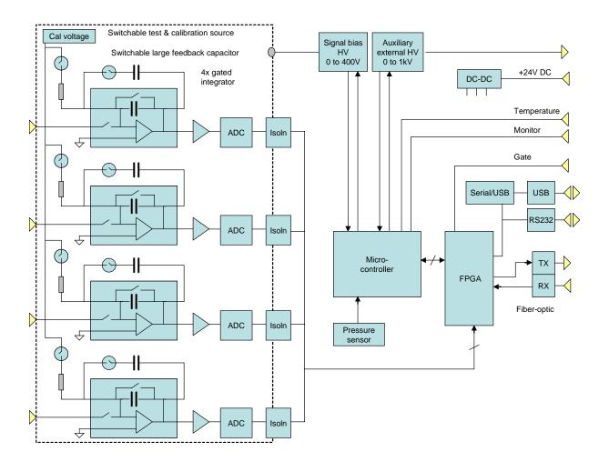
Figure 18. 1400 block schematic.
