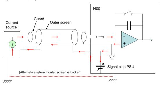
Figure 4. Path of measured current.
