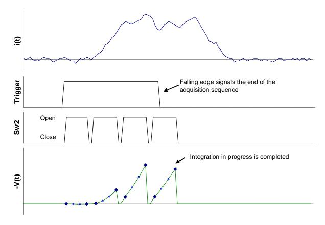
Figure 26. Example of an "external start/stop" triggered measurement sequence started by a rising edge and ended by a falling edge.
