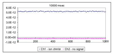
Figure 38. Separation of a 5 pA signal from background
