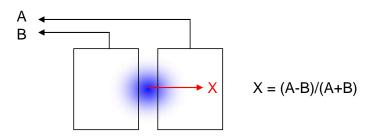
Figure 39. Single axis readout from a split sensor
