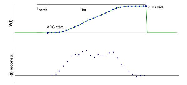
Figure 23. Reconstruction of a current pulse waveform from sub-integration samples.
