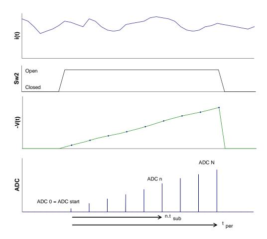
Figure 17. Data acquisition timing diagram. The plots are (from the top) illustrative input current waveform; integrator gate Sw2 state, integrator output with ADC sample points shown; ADC readings.
