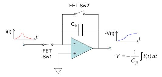
Figure 16. The basic gated integrator circuit.
