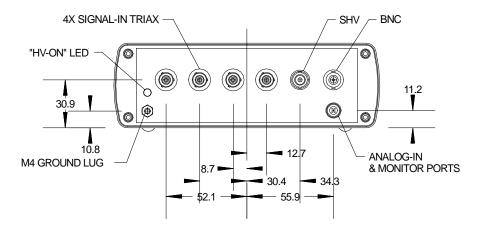
Figure 1. 1400 chassis end panels. Dimensions mm.
