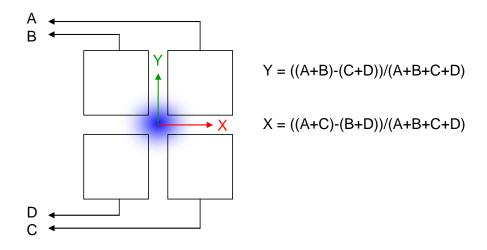
Figure 40. Two axis readout from a quadrant sensor
