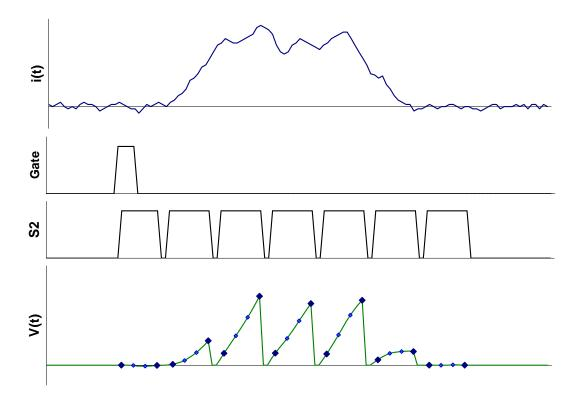
Figure 25. Example of an "external start" triggered measurement sequence started by a rising edge
