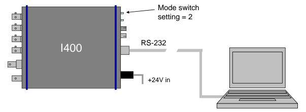
Figure 9. Direct RS-232 connection to the I400.
