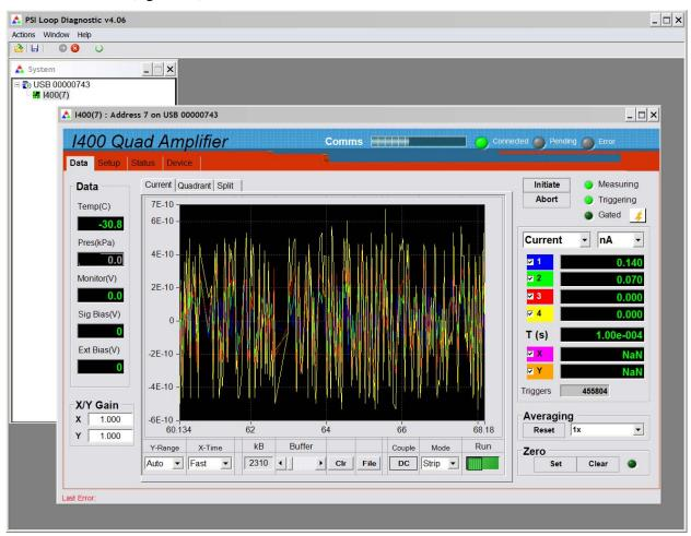
Figure 12. Data/current tab: I400 running with default settings, showing background noise.
