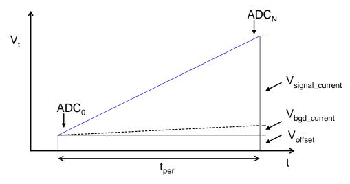
Figure 28. An integration showing signal and noise contributions to the final output.
