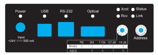
Figure 30. Rear panel showing controls and indicators
