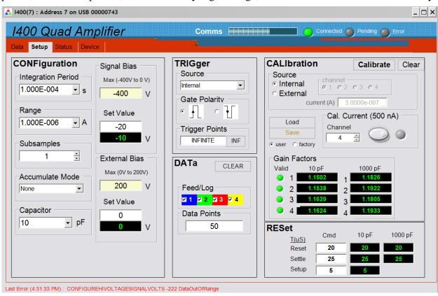
Figure 13. Setup tab: I400 running with default settings.
