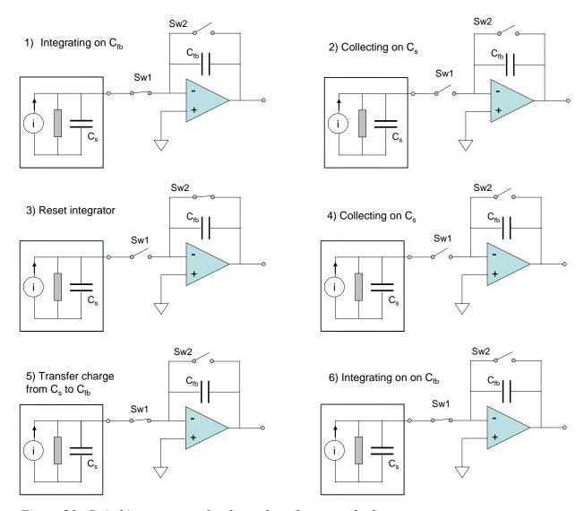
Figure 21. Switching sequence for the no-lost charge method.
