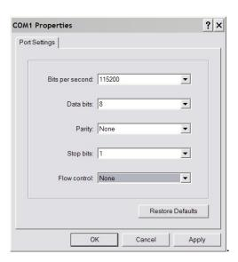
Figure 6. Hyperterminal COM port setup.
