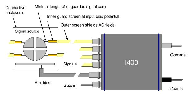
Figure 3. Schematic I400 installation
