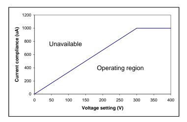
Figure 29. Current compliance of the high voltage supplies.
