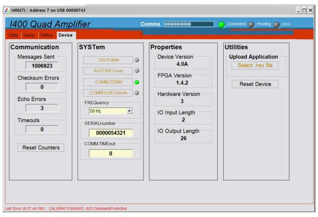
Figure 15. Device tab, showing firmware update utility controls.
