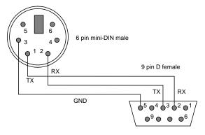
Figure 5. RS232 connection cable from the I400 to a PC serial port (DB9). Pins are shown looking at the face of the connectors.
