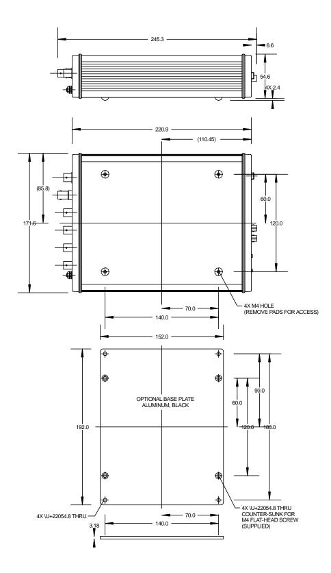
Figure 2. I400 case side and plan views (above) and optional mounting plate (below). Dimensions mm.
