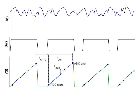
Figure 19. Timing diagram for continuous current monitoring. The deadtime for setup, reset and settle  $(t_{s-r-s})$  is shown relatively large.
