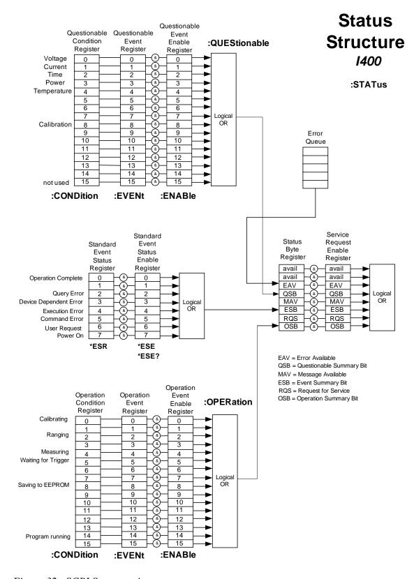
Figure 32. SCPI Status register structure
