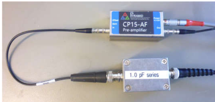
Figure 13 Setup for conversion gain calibration
