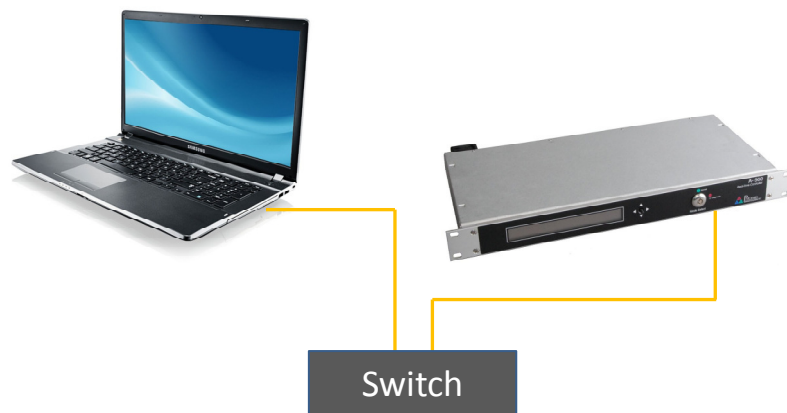
Figure 19. Network connection via switch.
