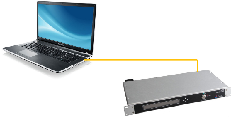
Figure 8. Direct patch cable connection from host computer to A560.
