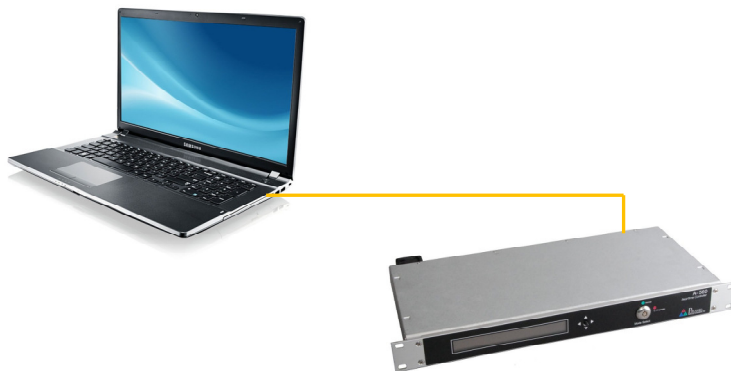
Figure 18. Direct Ethernet connection.
