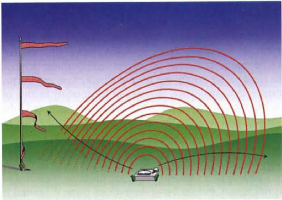
Figure 3: Wind shear, with upward and downward refraction upwind and downwind respectively, as illustrated by Professor Osborne Reynolds circa 1876.
