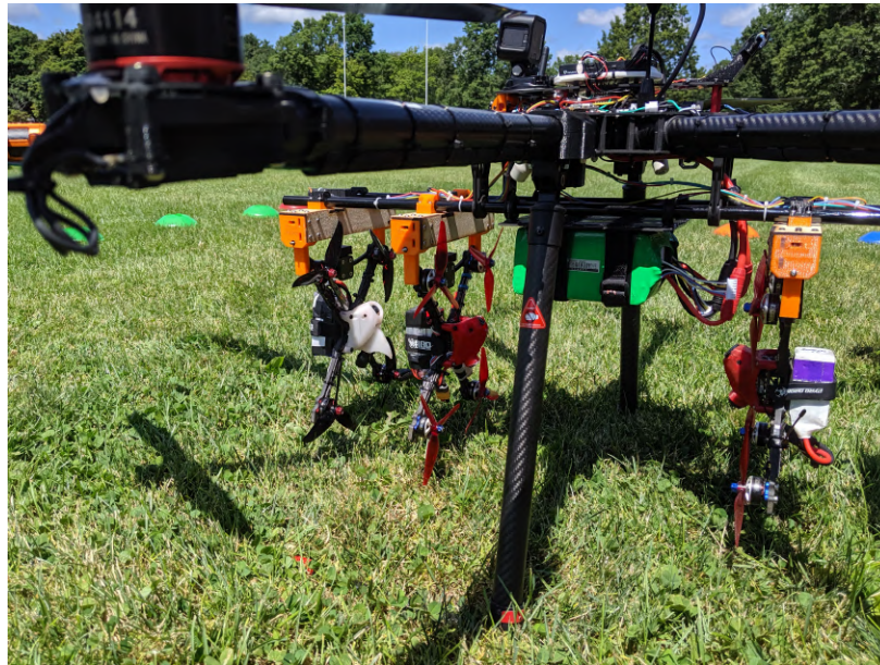
Figure 12: Octocopter with three FPV quadcopters for the initial test of Drop Mode
