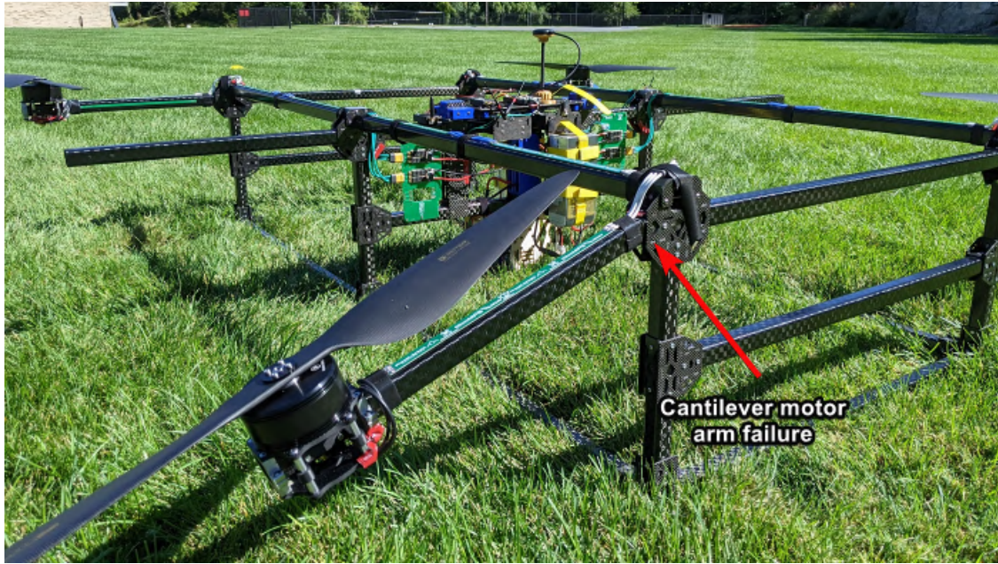
(a) Carrier Drone V1 failure of motor cantilever arm
