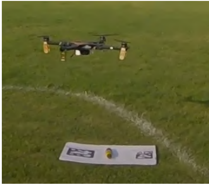
Figure 56: Swarm Drone performing a precision landing during testing
