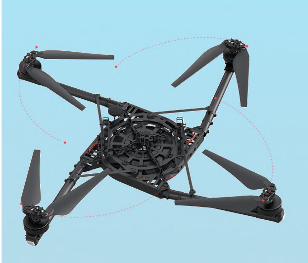
Figure 5: Industry airframe design example: Freefly Systems Alta X [5]
