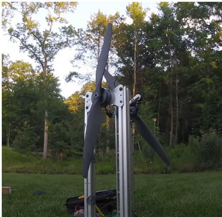
Figure 55: RCbenchmark S1780 Motor Thrust Test Stand with Coaxial Configuration
