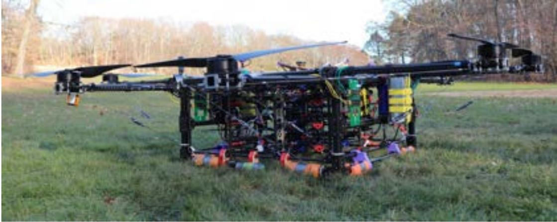
**(a) Side view: Carrier Drone loaded with 3 Swarm Drones on the ground**
