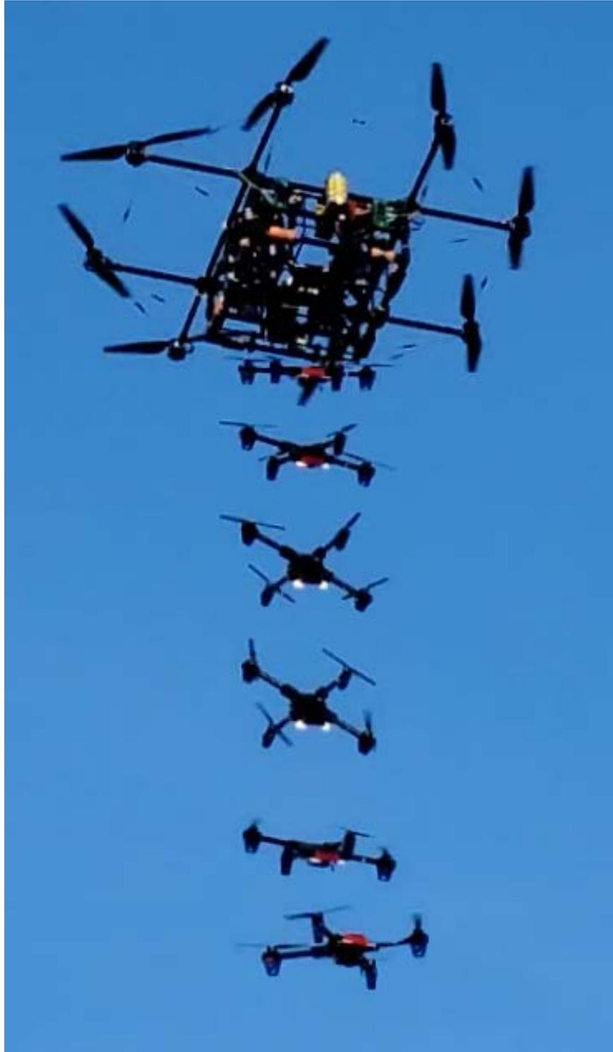
**Figure 96: Long exposure of the Swarm Drone deploying from the Carrier Drone**
