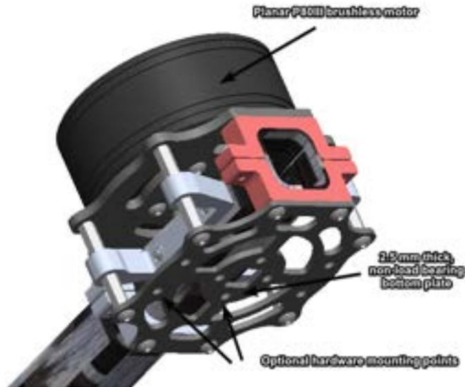
(a) Planar Motor Mount Configuration (CAD)
