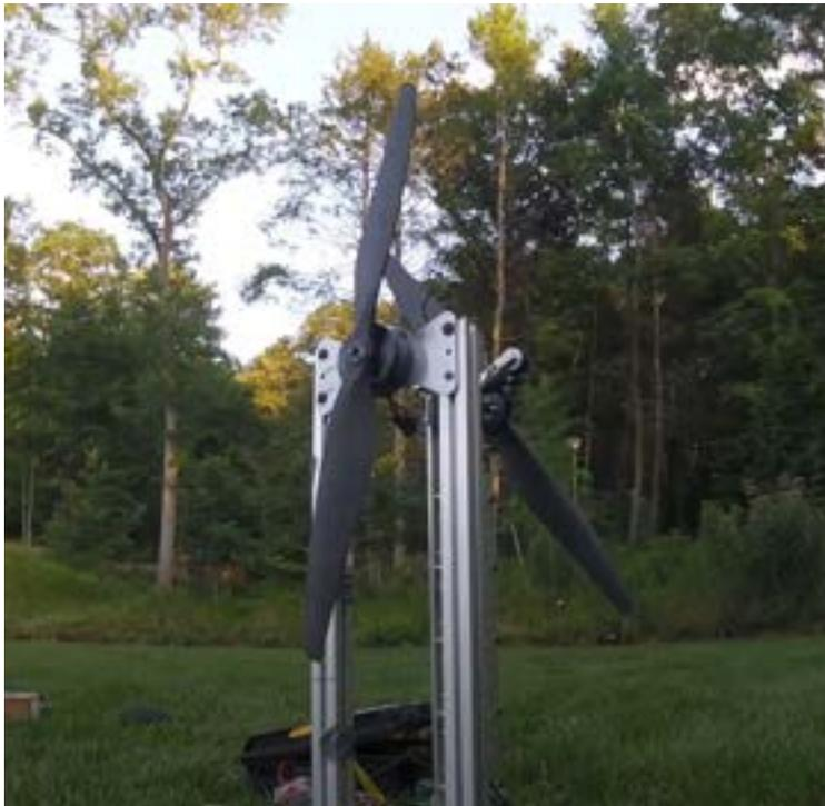
**Figure 77: RCbenchmark S1780 Motor Thrust Test Stand with Coaxial Configuration**
