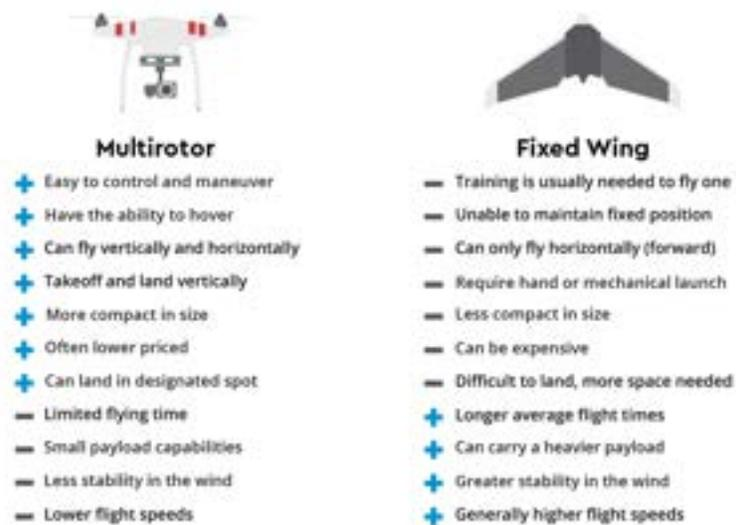
Figure 1: Multirotor vs. Fixed Wing Capability [1]
