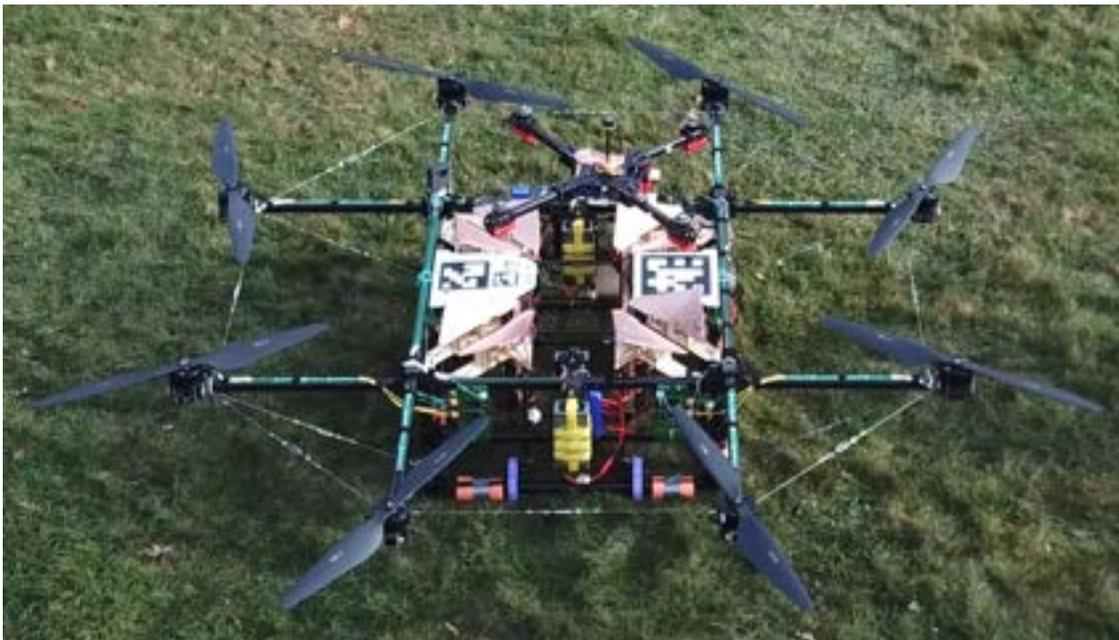
**Figure 80: Swarm Drone performing a precision landing on Carrier Drone**
