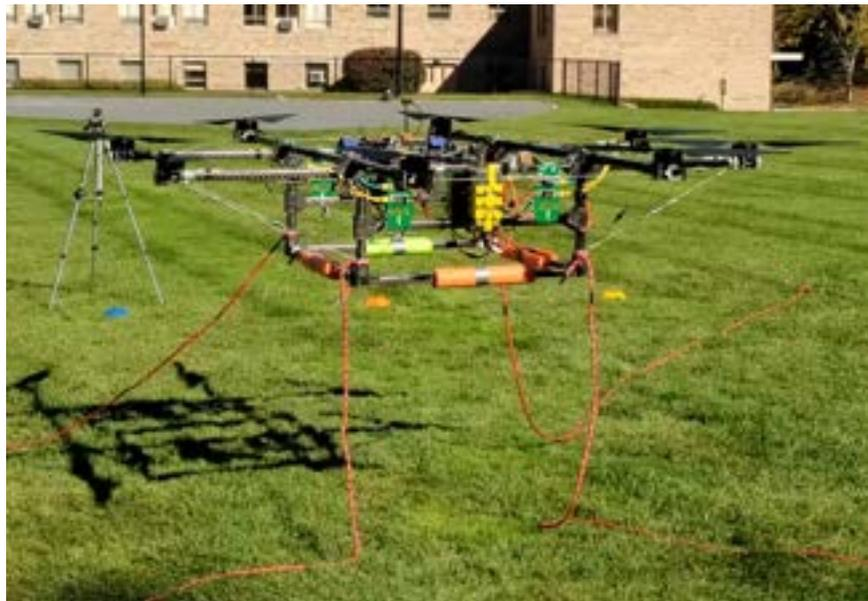
**Figure 90: Tethered Carrier Drone flight test**
