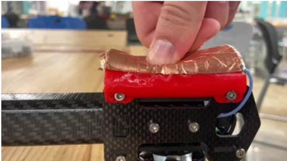
(b) Exaggerated example: compliant sensor compression
