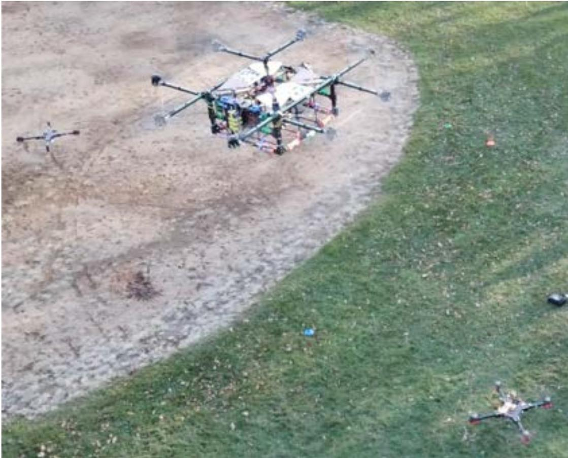
**Figure 93: Carrier Drone hovering with two Swarm Drones**
