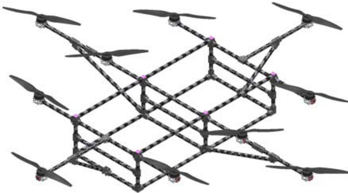
**Figure 26: Carrier Drone V2 CAD**
