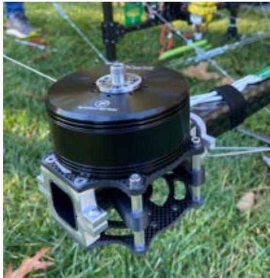
(b) Final Motor Mount on the Carrier Drone
