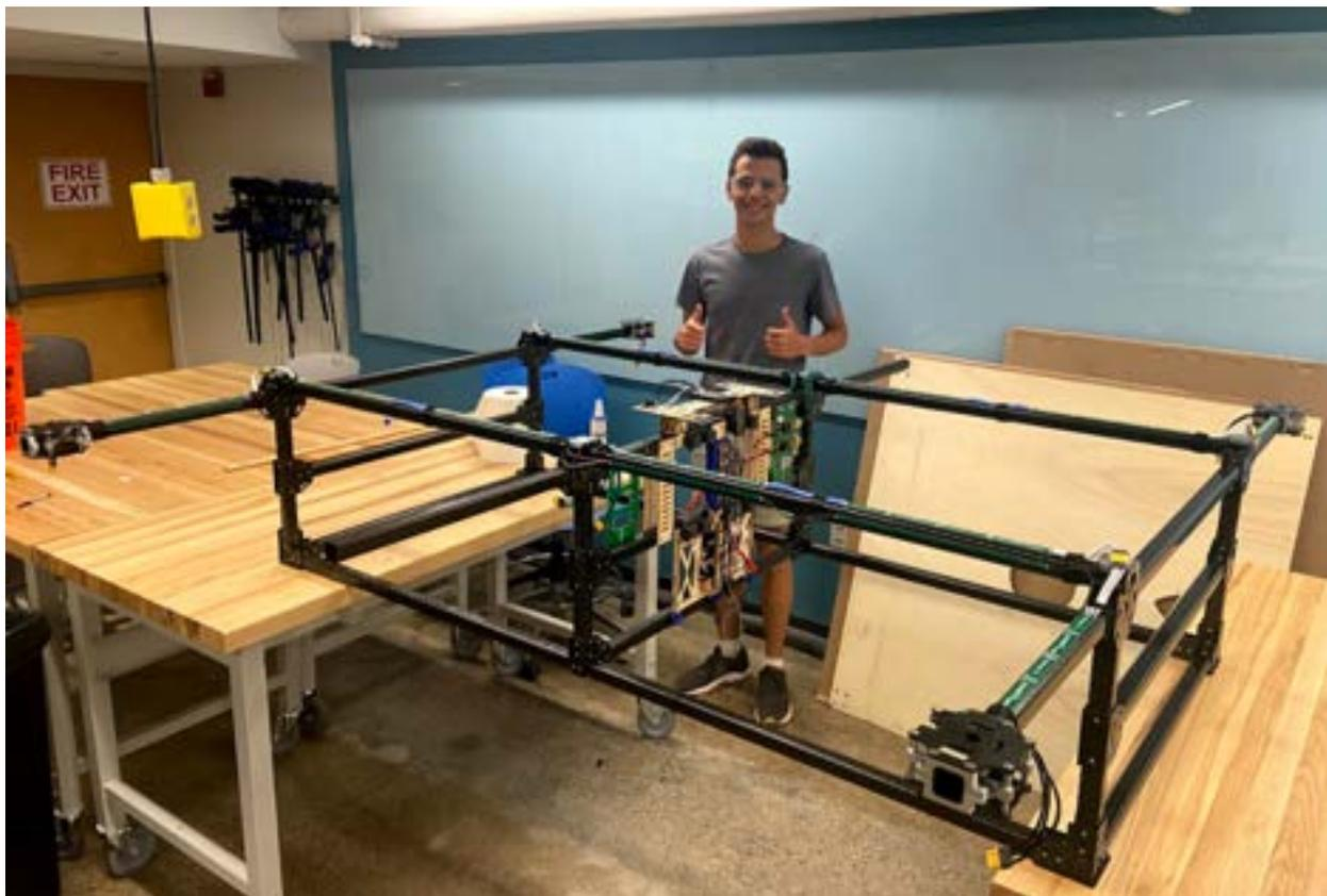
(b) Carrier Drone V1 Airframe Prototype
