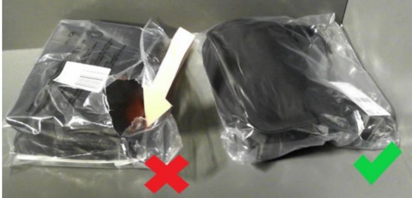
Problem: Damaged Polybag (shown by the orange arrow)
