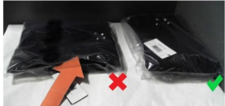
Problem: Open Polybag and hang tag outside (shown by the orange arrow)
