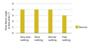
Background: During normal gait, the knee is flexed a few degrees at the beginning of the stance phase. This is done for reasons of shock absorption, stabilisation of the knee and forward progression.21 With most knee joints this is not possible and people step on a fully extended or even hyperextended leg.<sup>22,23</sup> With Genium PreFlex the knee is already flexed at 4° at heel strike and also allows controlled flexing of the knee during stance phase.
