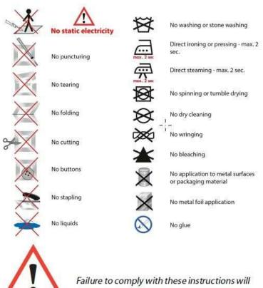
result in permanent damage to RFID tag
