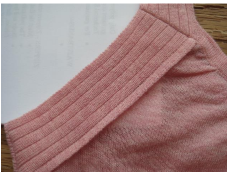
An example of modified all needle rib/flat back rib
