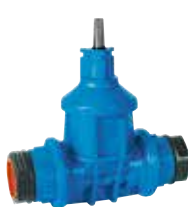
Series 16/90 Service connection valve with PRK couplings DN25-50 PN16 POM (Polyoxymethylene)
