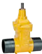
Series 46/64 Gate valve with short spigot ends DN50-300 PN16 Cast steel GP240GH External epoxy coating
