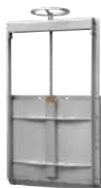
Series 772/61 Wall penstock Bi-directional up to and incl. 1200 x 1200 mm, in larger sizes bi- or uni- directional With non-rising stem Stainless steel AISI 304 200 x 200 mm - 2000 x 2000 mm
