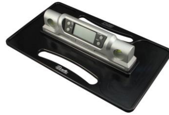
Figure 6: Official measuring device to check saddle inclination
