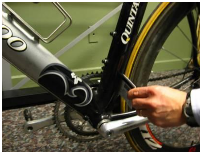
Figure 65: Insertion of a credit card between the wheel and frame to check that a fairing is not present
