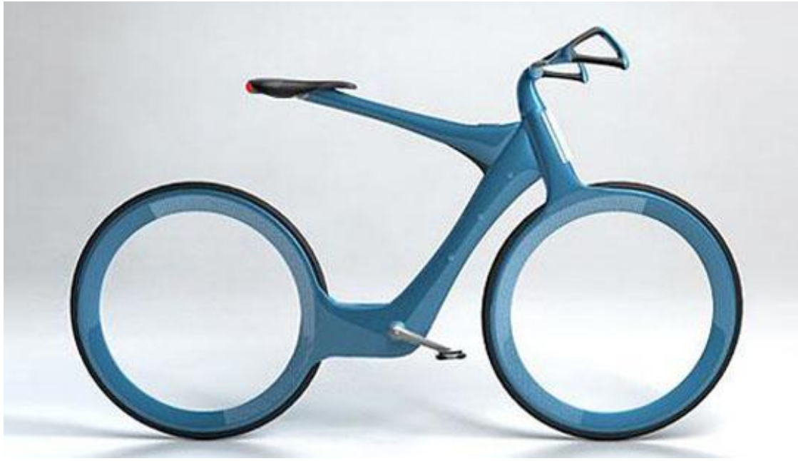
Figure 14: Example geometry of a bicycle that does not comply with UCI regulations
