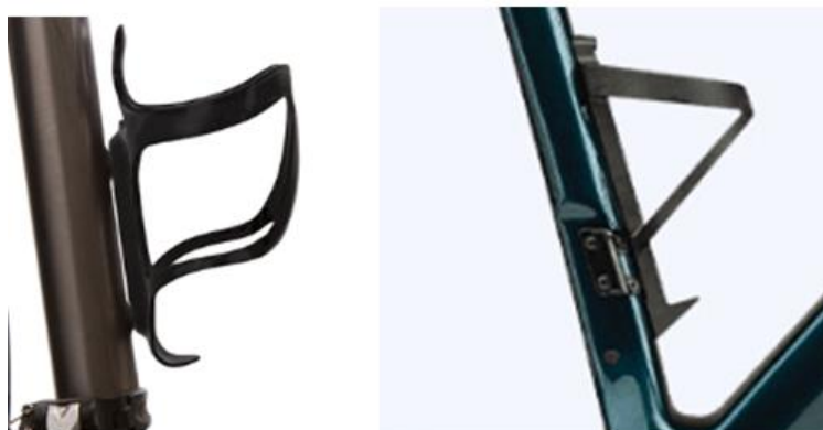
Figure 66 Illustration of a physical (left) and a visual (right) space between the bottle and the tube to which it is attached.
