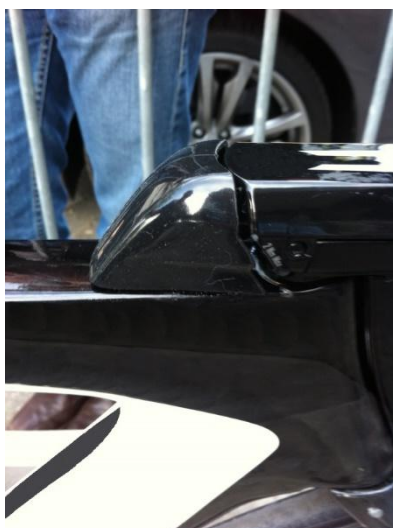
Figure 59: Cover added to frame to conceal brake cables
