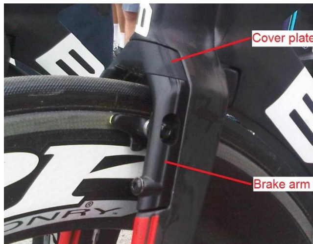
Figure 60: Brake integrated with the fork and fitted with a cover
