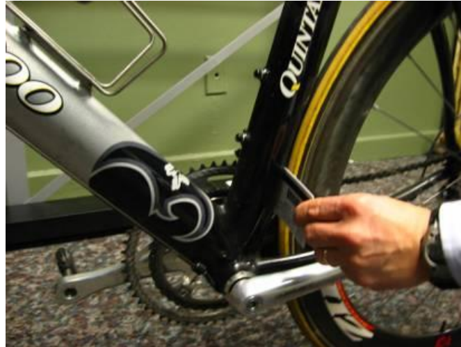
Figure 545: Insertion of a credit card between the wheel and frame to check that a fairing is not present
