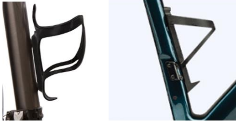
Figure 57: Illustration of a physical (left) and a visual (right) space between the bottle and the tube to which it is attached.
