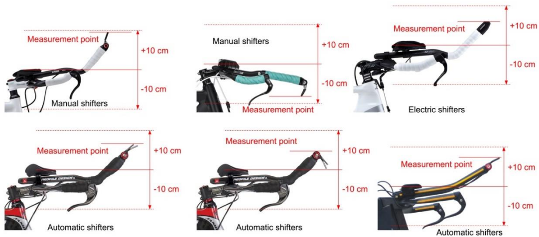
Figure 44: Points of measurement for the vertical limits of the fixed additional time trial extensions and any accessories
