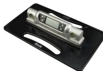
Figure 6: Official measuring device to check saddle inclination
