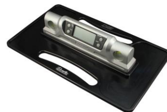
Figure 6: Official measuring device to check saddle inclination
