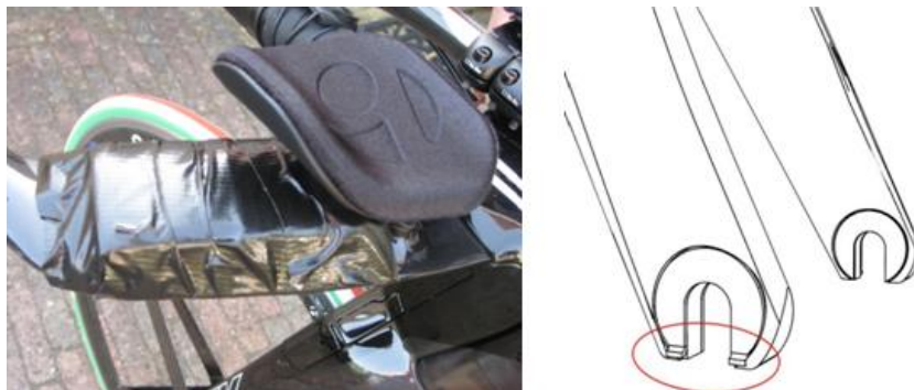
Figure 1: Examples of the prohibited modification of equipment (addition of tape, filing off fork drop-out safety lugs)
