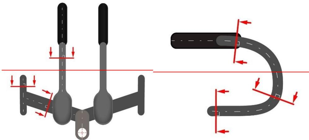
*Figure 57 : Illustration of the 3:1 rule application*
