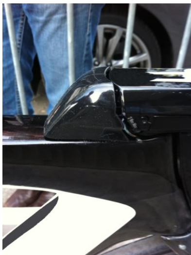
Figure 54: Cover added to frame to conceal brake cables
