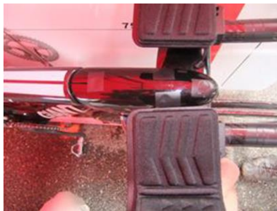
Figure 4: Illustration of the addition of the adhesive tape to cover bolts access
