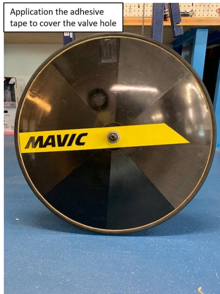
Figure 3: Example of application the adhesive tape on the Time Trial disc wheel
