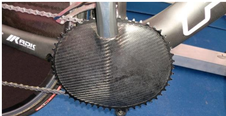
Figure 2: Example of the prohibited modification of equipment (the carbon cover added to the chainring)
