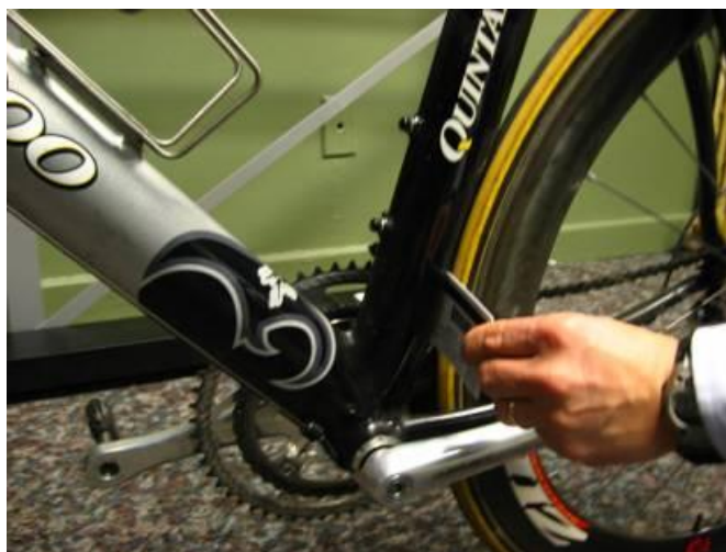
Figure 60: Insertion of a credit card between the wheel and frame to check that a fairing is not present
