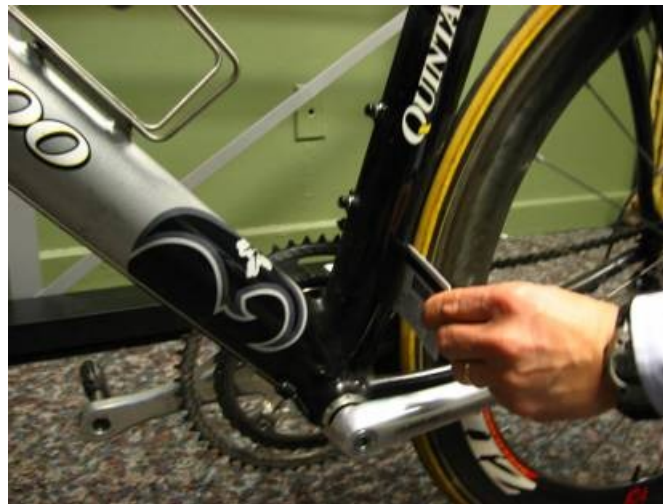
Figure 53: Insertion of a credit card between the wheel and frame to check that a fairing is not present
