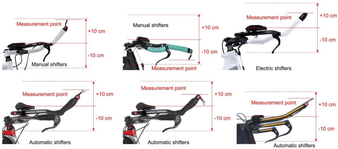
Figure 48: Points of measurement for the vertical limits of the fixed additional time trial extensions and any accessories
