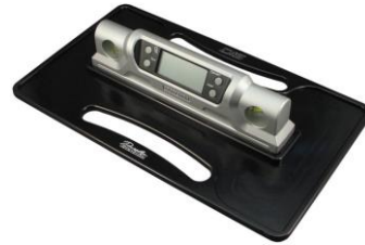
Figure 6: Official measuring device to check saddle inclination
