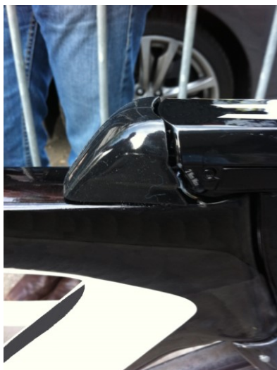
Figure 42: Cover added to frame to conceal brake cables
