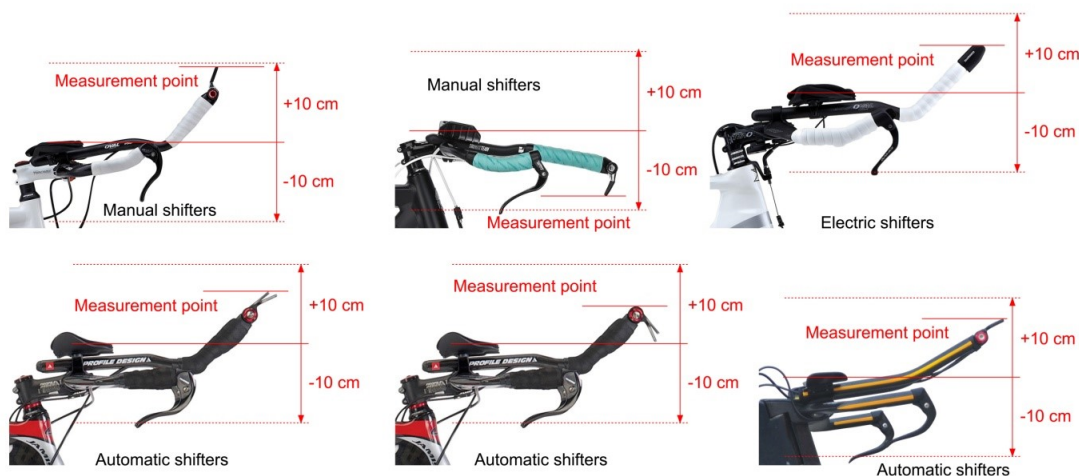
Figure 38: Points of measurement for the vertical limits of the handlebars extensions and any accessories
