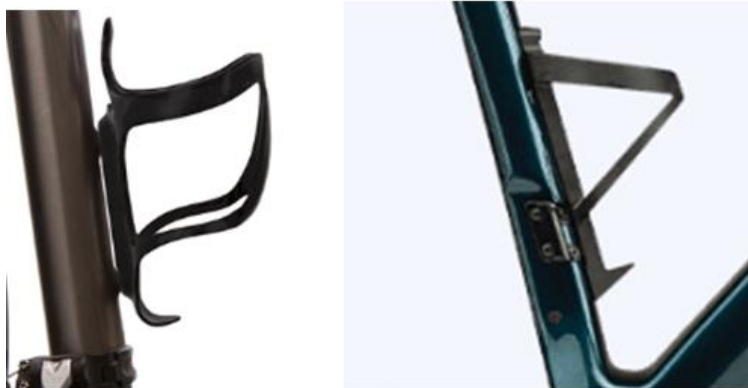
Figure 61 Illustration of a physical (left) and a visual (right) space between the bottle and the tube to which it is attached.
