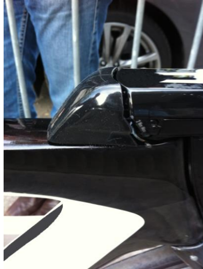
Figure 52: Cover added to frame to conceal brake cables
