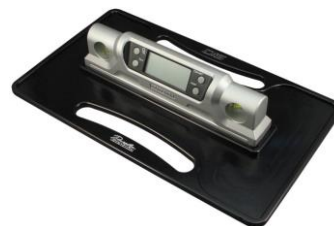
Figure 6: Official measuring device to check saddle inclination
