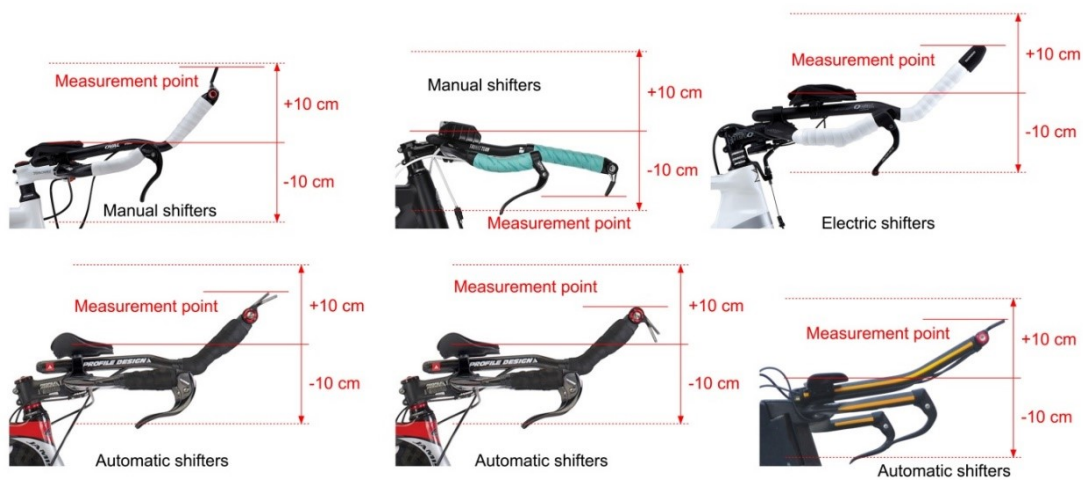
Figure 53: Points of measurement for the vertical limits of the fixed additional time trial extensions and any accessories
