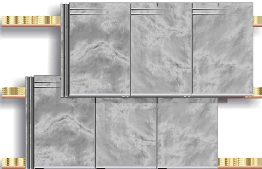
Tiles must be laid broken-bond and mechanically fixed according to specifications
