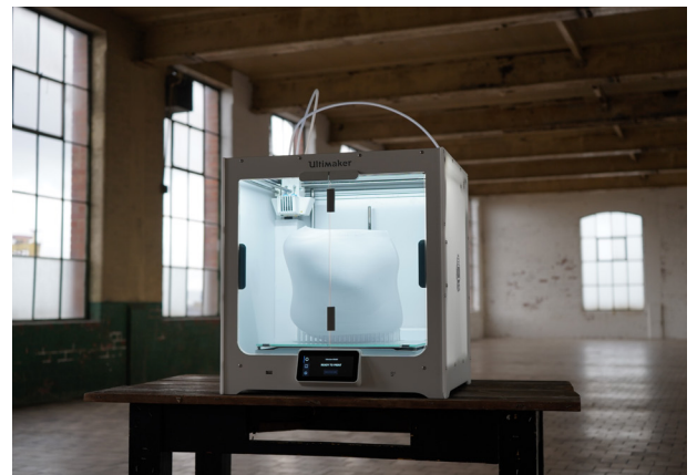
Segment of the 3D printed Ocean Orbs printed on an Ultimaker S5.
