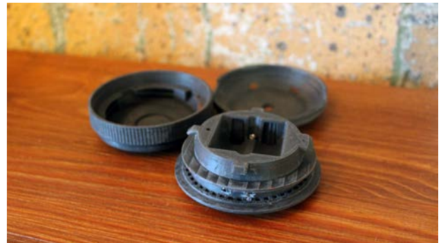
Functional prototypes created with the Ultimaker 3 allow NoiseAware to test features like design, acoustic performance, and RF transmission for immediate feedback.
