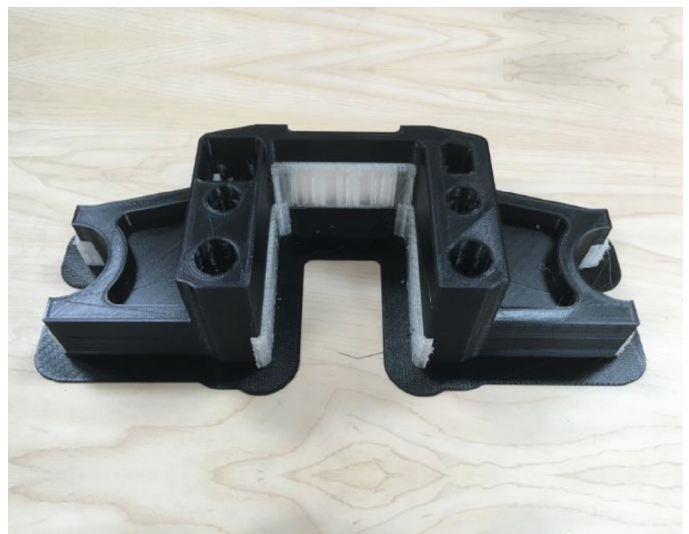
The ability to design and 3D print parts means they can control infill densities and wall thickness for control over part mass and weight.
