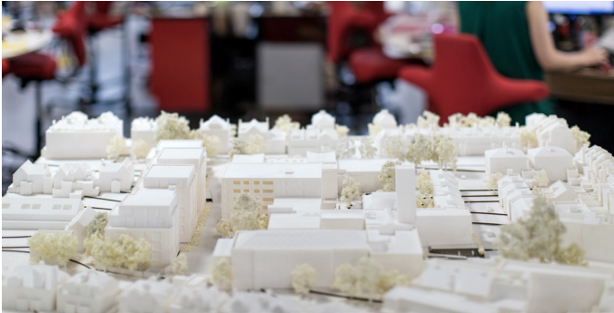
Large context models are 3D printed in-house and to scale and can be produced within a week. Similar models fabricated from timber were outsourced and took up to six weeks
