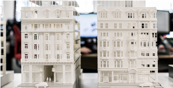
Using a variety of post-processing techniques, like spray painting and laser cutting, model-makers can further enhance 3D printed structures to produce high quality presentation models
