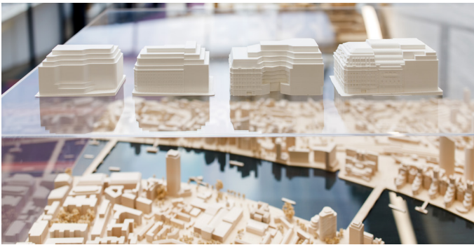
Every employee is inducted to use the Ultimaker 3D printers, enabling them to produce rapid iterations or ‘3D sketches’, which test the design constraints of the site
