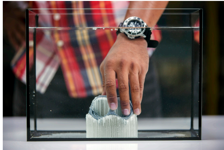
PVA (the white material) dissolves in water
