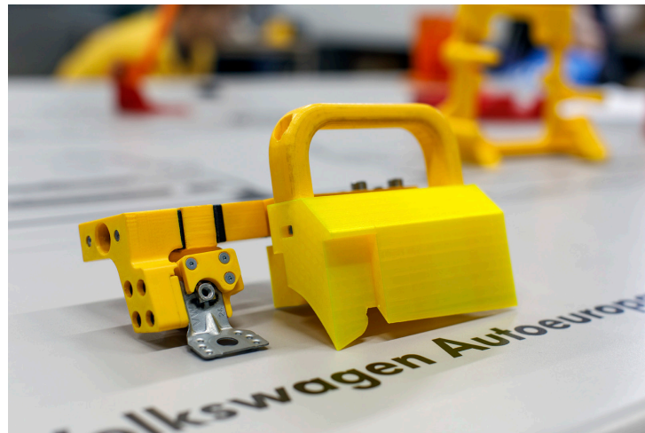
A 3D printed tool assembled from multiple parts
