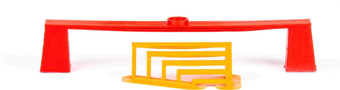
The effects of bridging on different sized prints
