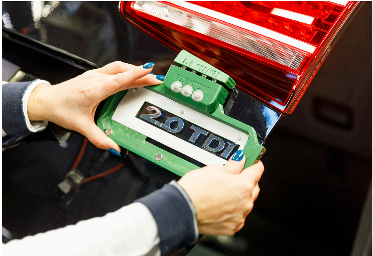
Volkswagen Autoeuropa uses Ultimaker printers to create tooling for the production line
