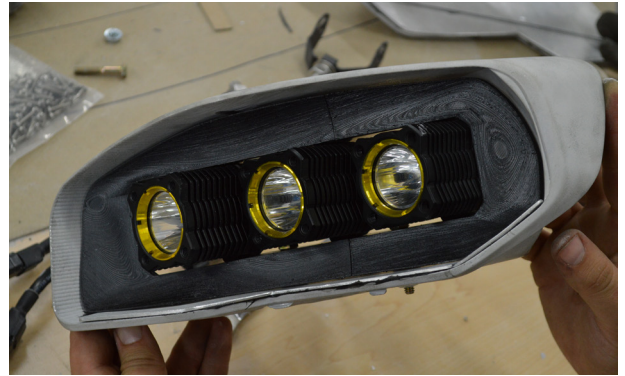
Assembling and testing customized 3D printed Ford Fiesta ST headlights.
